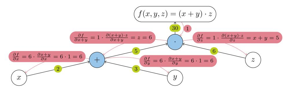
Figure 1 Reverse mode automatic differentiation f(x, y, z) = (x + y) \* z on x=2, y=3, z=6 [2]
