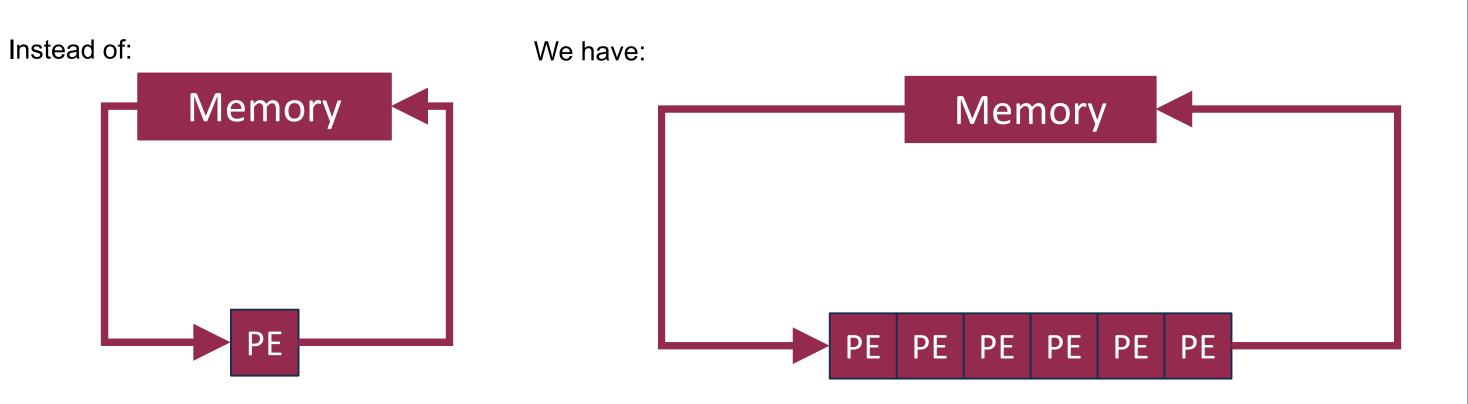
Figure 4 Illustration of a systolic array in comparison to a non-systolic architecture. Adapted from [3].
