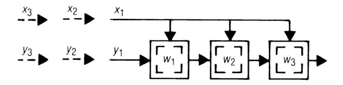
**Figure 5** Systolic array with cells. Input  $(x_i)$  is broadcasted to the cells. Weights  $(w_i)$  stay. Results  $(y_i)$  move systolically. [3]
