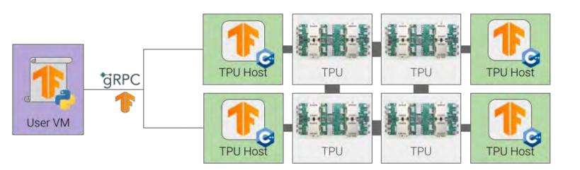
*Figure 8* Illustration of the TPU Node architecture. No direct access to the TPU Hosts is possible. [2]
