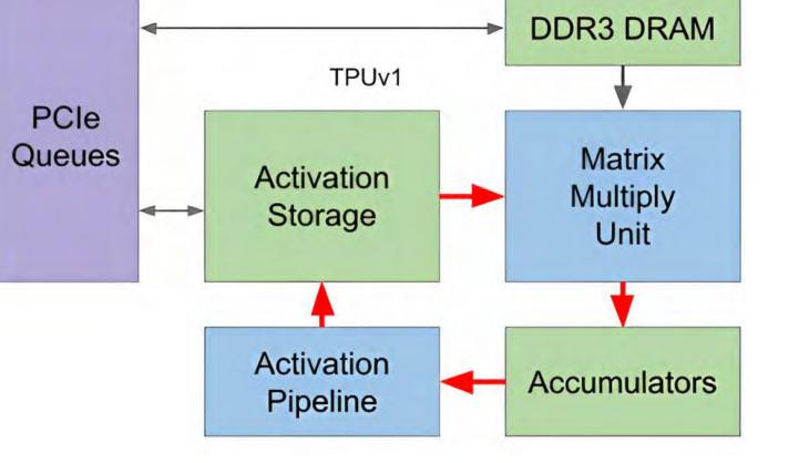
Figure 3 TPU Block Diagram. [4]
