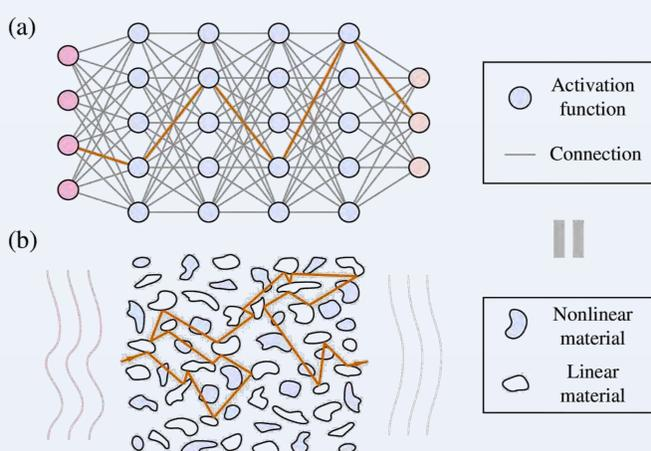
**Figure 2.** (a) Conventional ANN architecture. (b) Proposed Nanophotonic Neural Medium. [3]
