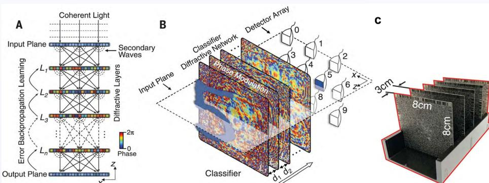
**Figure 1.** (A) multiple transmissive layers of D2NN. (B) Trained layers of a classifier NN. (C) 3D printed layers of the classifier. [2]
