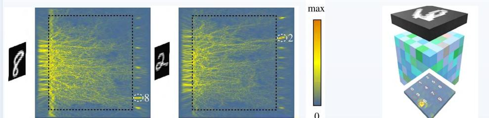
**Figure 5.** (left) Light field distribution in the trained NNM. (right) 3D NNM consists of multiple NNM layers. [3]
