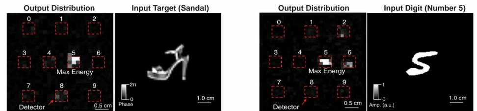
**Figure 3.** The input and output images of the 3D-printed D2NN for a sandal input (Fashion-MNIST class 5), and a handwritten input of "5". [2]
