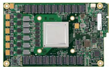
Figure 1 TPUv1 Printed Circuit Board. [5]
